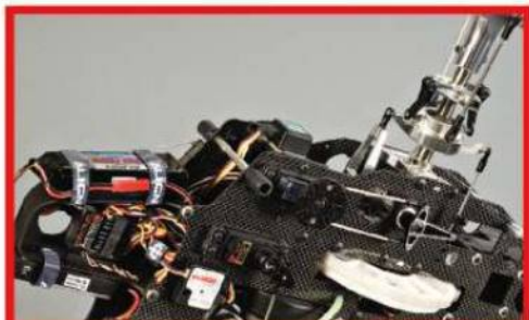
In viewing a CCPM arrangement next to a Mechanical setup as shown here, the differences are very apparent. Notice on the mechanical setup how each servo is connected to a single movement of the swash while the CCPM bird uses all three to do the job.
